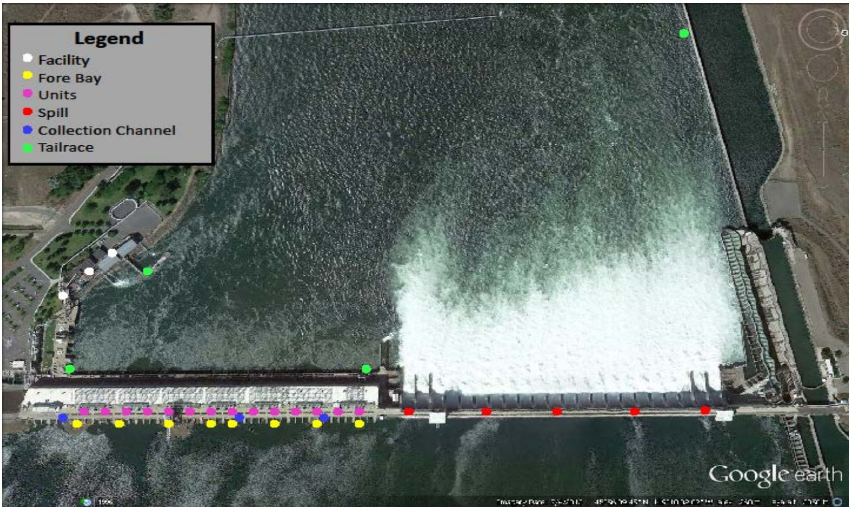
Figure 1. Placement of temperature data devices at McNary Dam, 2013* *Picture was taken July 4, 2013
